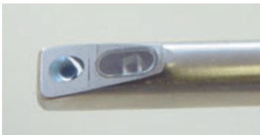
The Wolf product range of swivel prism borescope has now been extended to the world's smallest diameter of 5.5 mm (by Jan. 2009).
